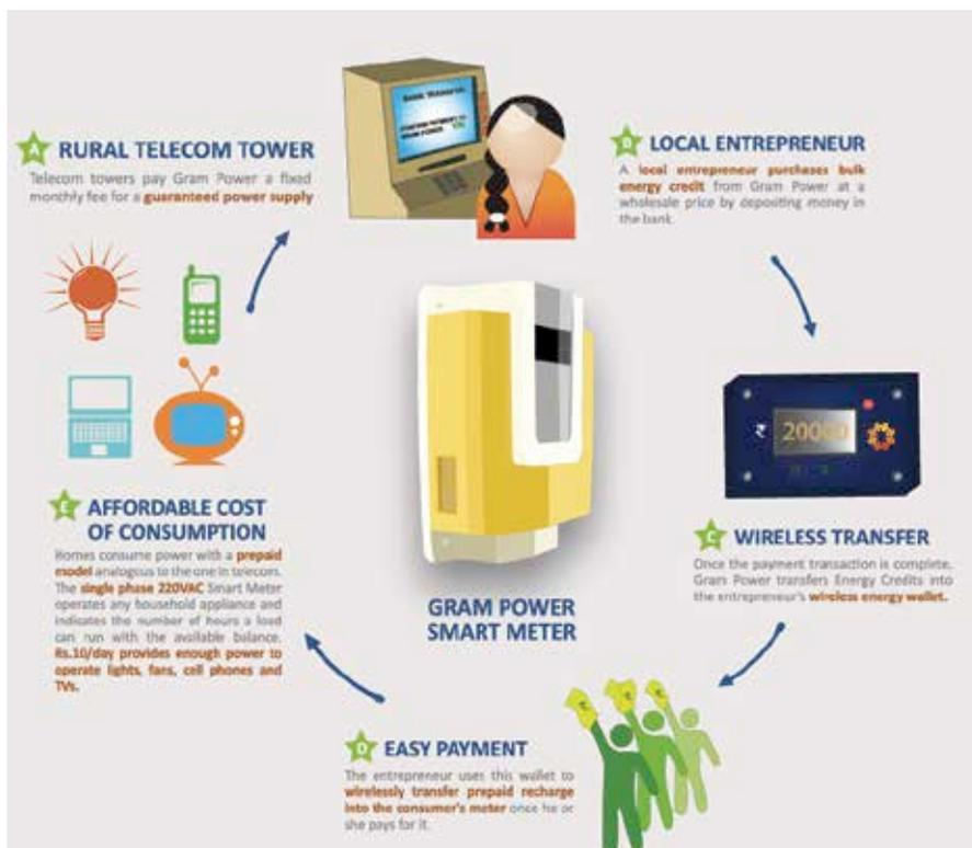
This infograph neatly explains how Gram Power operates. It's pretty much like recharging one's cell phone balance, that's how easy it is to top-up your electricity quota.
